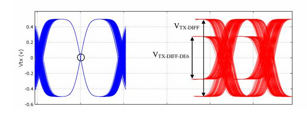
Figure 55. CLK to CAD data eye with some transmit jitter
