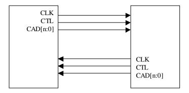
Figure 1. HyperTransport<sup>TM</sup> I/O Link
