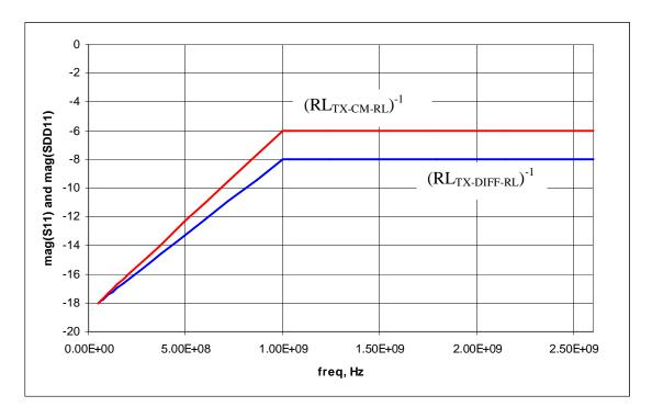
Figure 50. Transmit return loss mask
