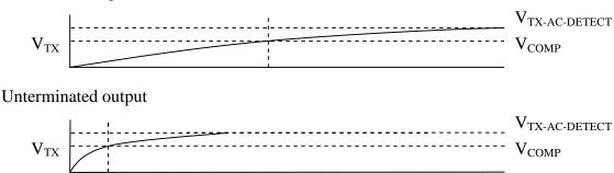
Figure 19. AC Detect Timing
