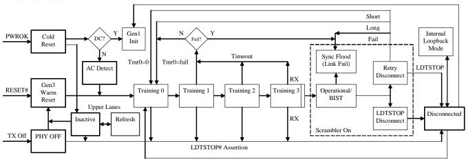
Figure 17. Link State Diagram
