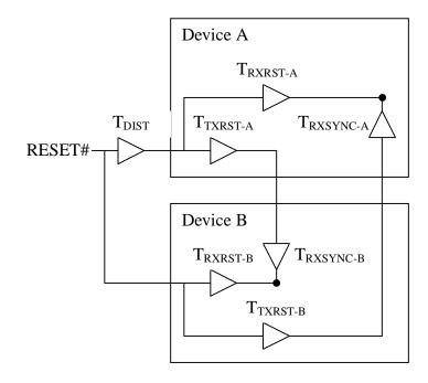
$T_{RXRST}$  – The delay from assertion of RESET# at the device pin to when inputs are ignored at an internal state commit point. < $T_{RXSYNC}$  recommended.
