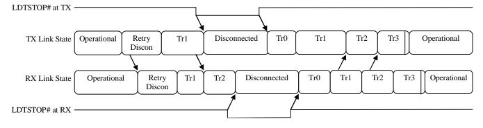
Figure 20. Example LDTSTOP Disconnect Sequences
