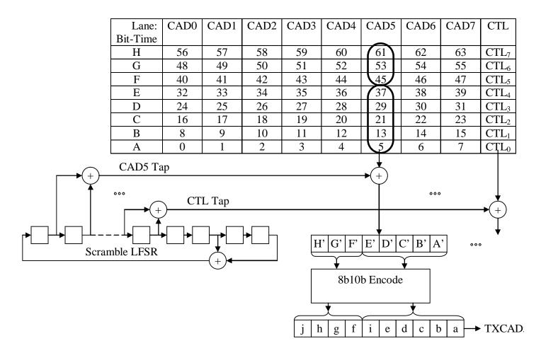
Figure 4. Gen3 Transmitter Order of Operations
