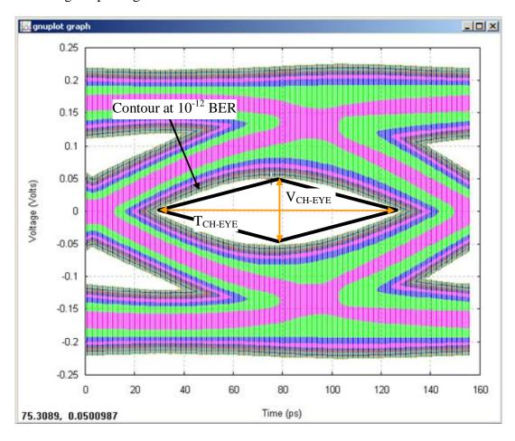
Figure 57. Channel compliance eye diagram
