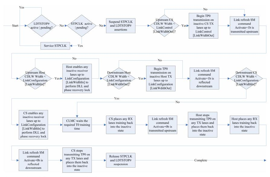
Figure 12. CLMC Sequencing Diagram for CILR
