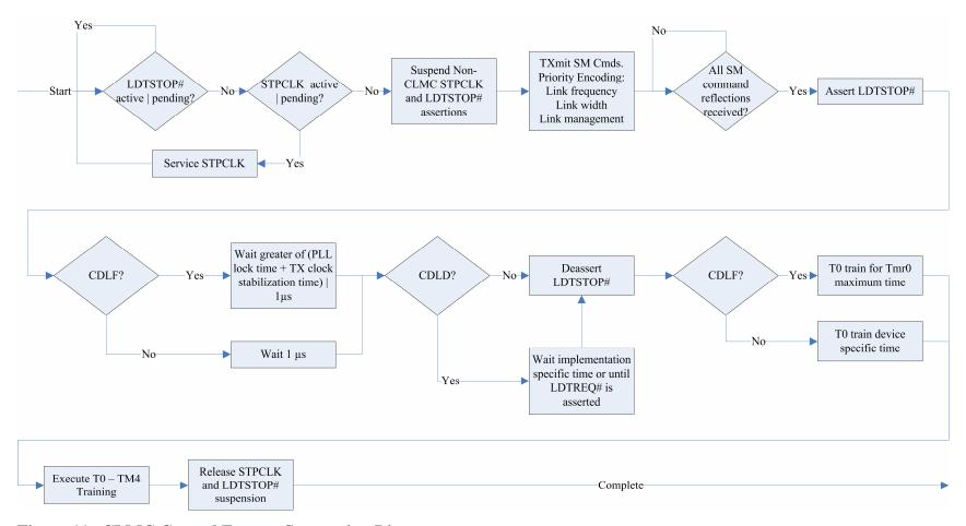
Figure 11. CLMC Control Feature Sequencing Diagram
