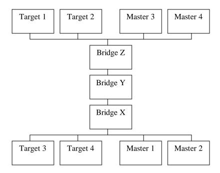
Figure 26. Example PCI System
