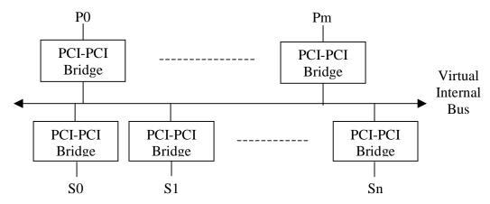
Figure 29. Logical Model of a Switch
