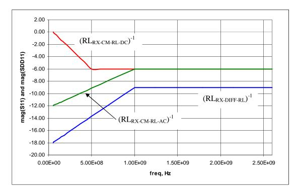
Figure 58. Receiver return loss mask
