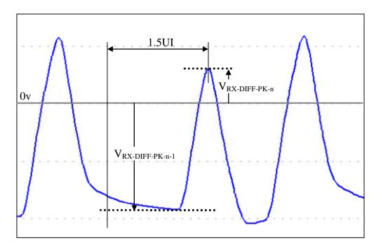
Figure 61. Receiver adjacent bit ratio
