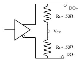
Figure 31. DC Output Reference System Load
