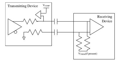
Figure 18. AC Detect Circuit
