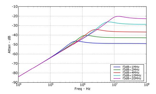
Figure 49. System reference clock jitter rejection
