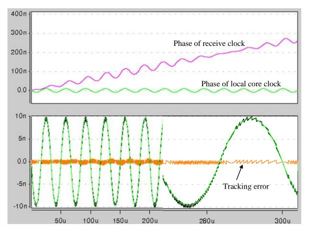
Figure 65. Phase tracking across receiver sync-fifo
