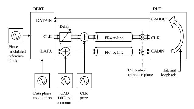
Figure 63. Receiver input compliance test setup
