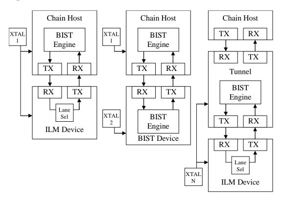
Figure 22. Link Test Topologies
