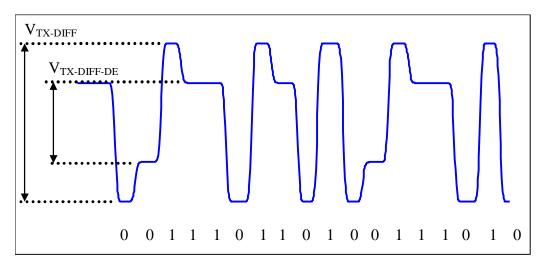
Figure 51. Differential transmitter post-cursor de-emphasized waveform
